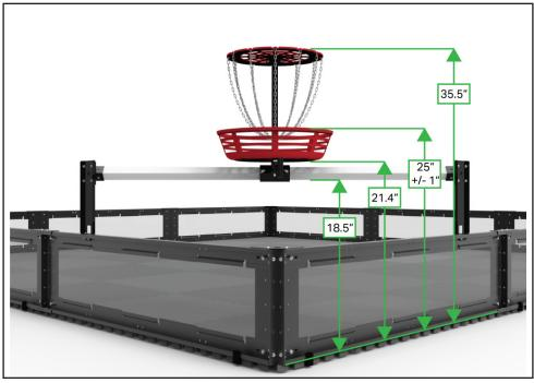
Figure 20: Vertical dimensions of the High Goal
