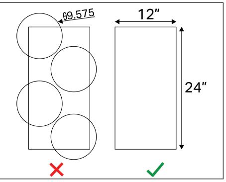
Figure 23: Custom plastic parts must fit within a single 12" x 24" sheet of plastic.
